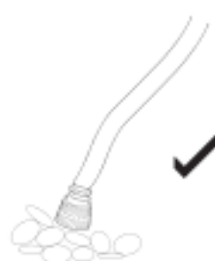
Fig 6 Protecting the suction filter from unnecessary debris
