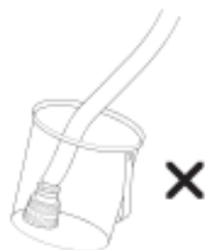
Fig 7 Protecting the suction filter from unnecessary debris
