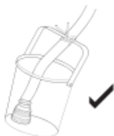
Fig 7 Protecting the suction filter from unnecessary debris
