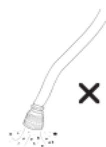
Fig 6 Protecting the suction filter from unnecessary debris
