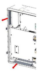
④ Insert new air filters of the same specifications into the air inlet and outlet respectively;
