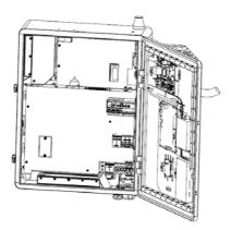
② Use an electric screwdriver to remove the inlet and outlet air duct cover and its mounting screws (M4x16).
