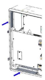
⑤ Install the side cover plate and lock the screw (M4×16). The reference torque of screw tightening: 16kgf. cm;
